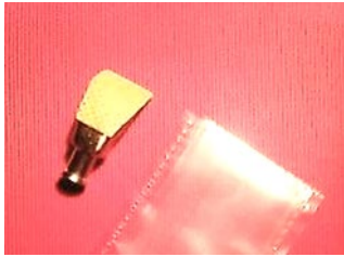
Fig. 1. Hooked – formed applicator with a heat-insulating nozzle on the back surface, an individual polyethylene cap
